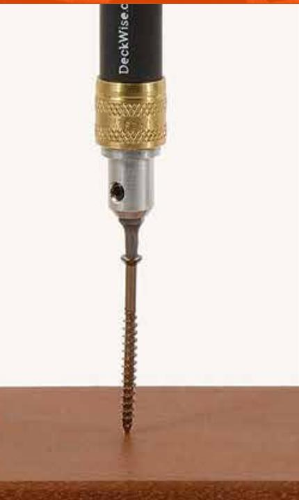
The **DECKWISE® HTSS™** (Heat-Treated Stainless Steel) deck screws offer our specially engineered four-sided tips with a serrated thread design to minimize board splitting or splintering, even when screwing near the edge.
