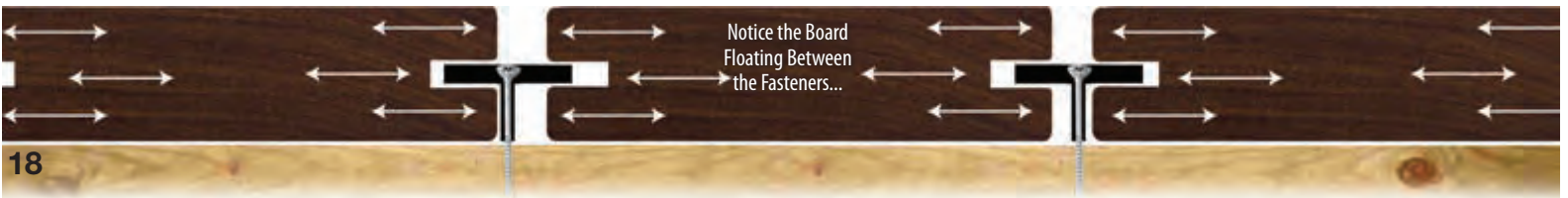
Shown Above: Ipe (Brazilian Walnut) Hardwood decking installed with hidden deck fasteners secured straight down.
